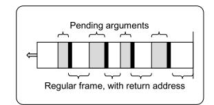
Figure 4. Stack layout for push/enter
