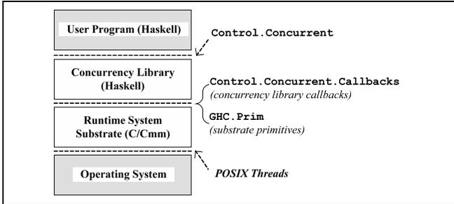
Figure 1: Components of the new RTS design
